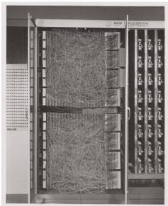
Frank Rosenblatt's Mark I Perceptron machine was the first implementation of the perceptron algorithm. The machine was connected to a camera that used 20×20 cadmium sulfide photocells to produce a 400-pixel image. The main visible feature is a patchboard that allowed experimentation with different combinations of input features. To the right of that are arrays of potentiometers that implemented the adaptive weights.
