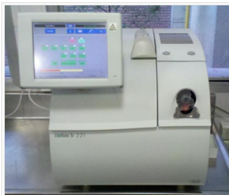
Figure 1: Blood gas analyzer. Photo source https://en.wikipedia.org/wiki/Arterial_blood_gas . This machine is used to run arterial blood gas (abg) tests on blood samples taken from patients. This test measures gases dissolved in blood, and is an important diagnostic tool in critical care and pulmonary medicine.
