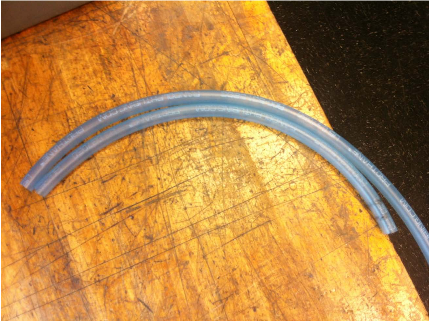
□ Fig. 4.17. Polyurethane Tubing . Here is the terrible Polyurethane tubing that proved too stiff to be used with our peristaltic pump. Unfortunately, no picture of the heaven-sent Tygon tubing was taken.
