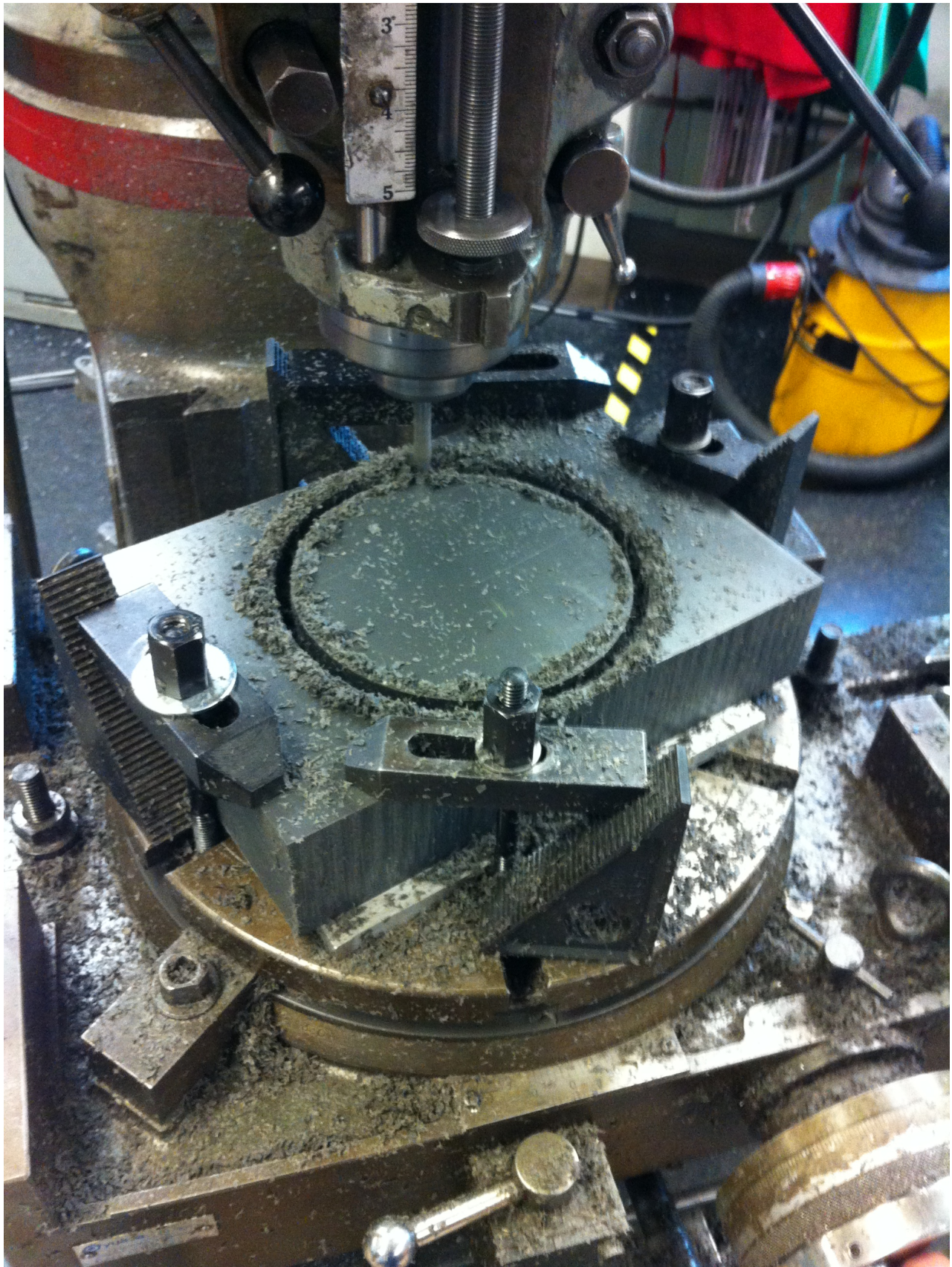
□ Fig 4.1. Machining the Back Arch 1. This image shows me working on drilling the circular part out of the back arch.
