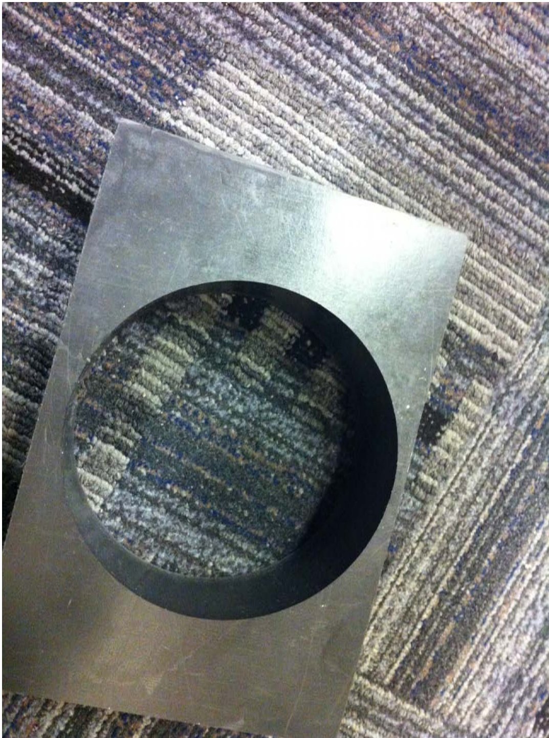
□ Fig 4.3. Machining the Back Arch 3 . The piece will be shaved down on the top and bottom until I break into the inner circle and thus have a relatively thin point as desired in the part drawings.
