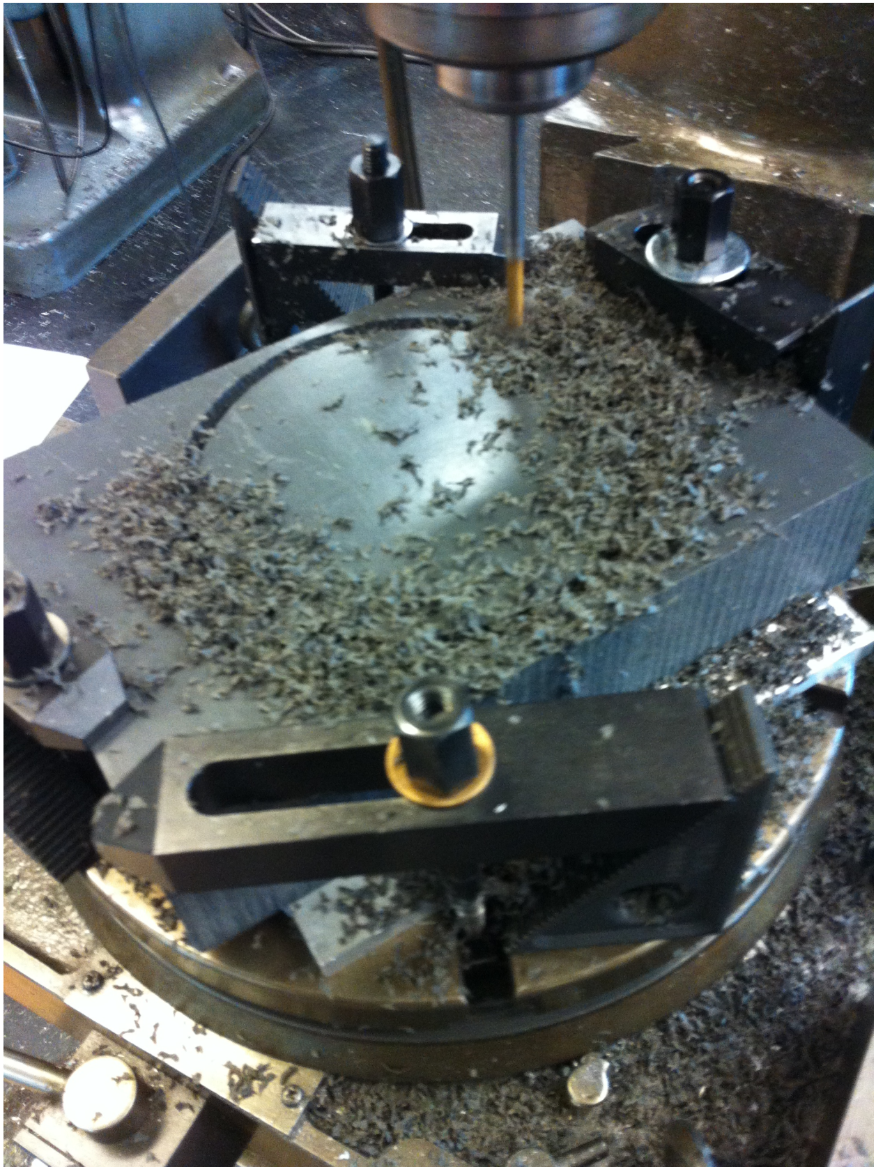
□ Fig 4.2. Machining the Back Arch 2. As you can see, this block is huge, so this process takes quite a bit.
