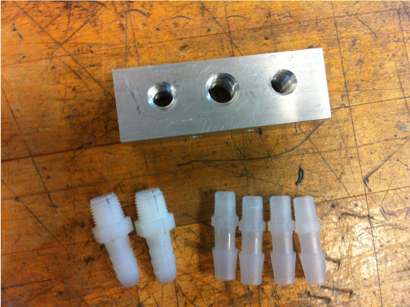
□ Fig 4.10. Fitting Jig 2 . Note the bigger hole drilled in and threaded in order to accommodate the larger spare tube fittings we found.
